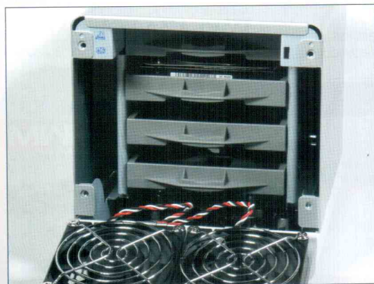
While the hard disk drives are all hot-swappable, accessing drive trays is a bit challenging despite the flip-open rear panel
