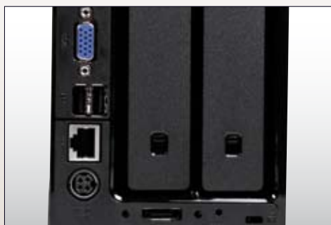
The rear interface offers plenty of expansion possibilities and functionalities with both an eSATA port and two USB ports
