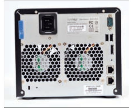
At the back of the unit you will find two exhaust fans that draw hot air out to ensure efficiency cooling system.
