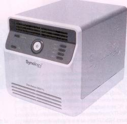
use the DS411j as a web and email server and even as a repository for IP camera footage. It can also download files from the web or BitTorrent. Confusingly, the option to restrict which users can use this download manager is in a separate Applications Privileges control panel.
